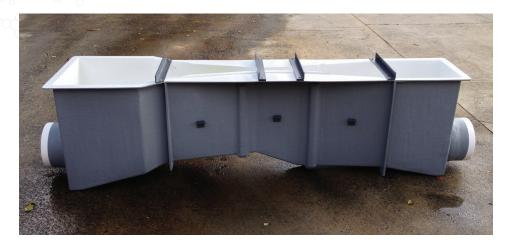
End adapters are specially shaped transitions that are molded or secured to the inlet and outlet ends of flumes to connect then to inline piping so that flow can be accurately measured.
