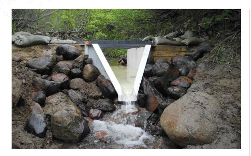
The 1930's saw the development of a simple flume to measure run-off from small plots and experimental catchments by the Soil Conservation Service, U.S. Department of Agriculture. The H flume, so called as it was the eighth design in a series starting with "A", combines the sensitivity of a sharp-crested weir with the self-cleaning properties of a flume.
