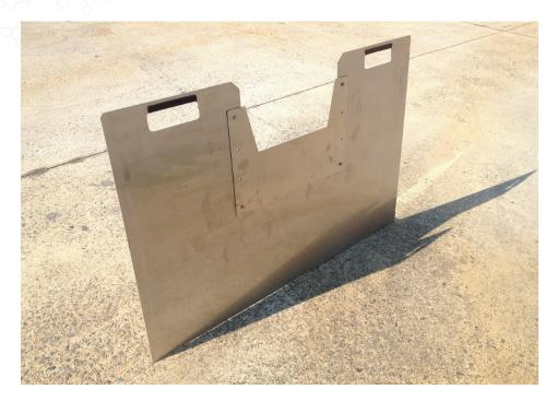
Portable Thin-Plate Weirs Plates from Openchannelflow offer an economical and flexible method of measuring open channel flows in natural channels.
