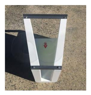
Unlike the Parshall flume, the Montana flume has a flat floor, with no drop to accelerate the flow.
