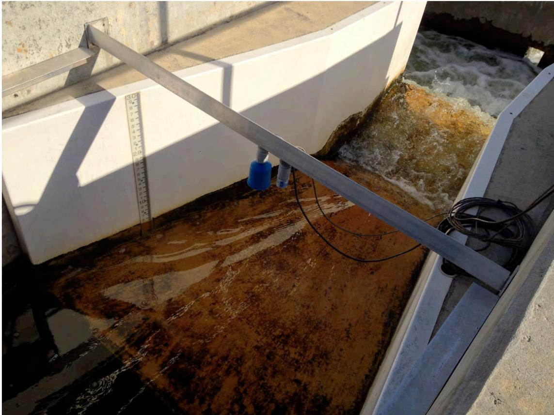
Standard Openchannelflow staff gauges are marked in centimeters on one side and feet / tenths / hundredths of a foot on the other. Custom gauges are also available, usually graduated in flow on one side and level on the other.
