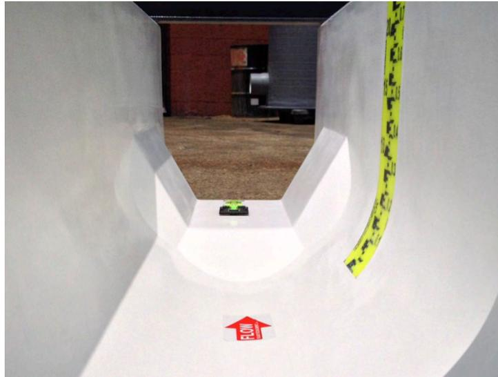
When using a staff gauge on a non-vertical surface it is important to know if the reading is corrected or uncorrected. For non-vertical applications, Openchannelflow indicates the primary device that the gauge has been designed (calibrated) for.
