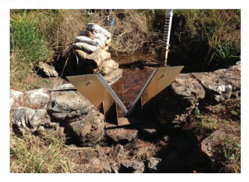
Portable thin-plate weirs offer an economical and flexible method of measuring open channel flows in natural channels.
