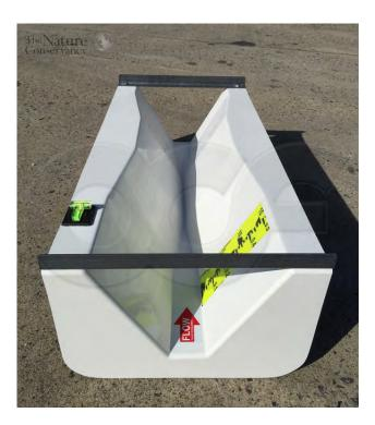
From above, the floor of the flume is wasp-waisted with the narrowest part the throat section of the flume.
